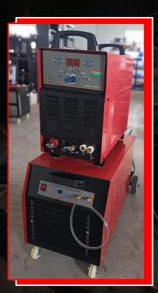
SWISS PULSE TIG 500 is an IGBT based inverter welding power source with in-built HF unit, cooling unit and water cooling torch for continuous welding applications.
